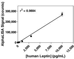
The data was generated using a white Optiplate-384 microplate and an EnVision-Alpha Reader 2102.
