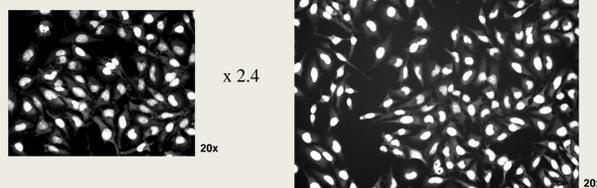
Fig. 2 The custom optical design, with resolution matched to the camera pixel size, enables you to image a 2.4 fold larger area (right) with every objective than compared to a standard microscope (left).
