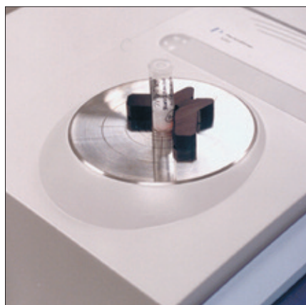
Figure 1. A powdered sample in its original glass-sampling jar is simply placed on top of the NIR sampling interface.
