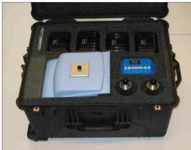
Figure 2. Kit includes Spectrum 100 sample pod, reflectance standards, supports for large panes and protective case.
