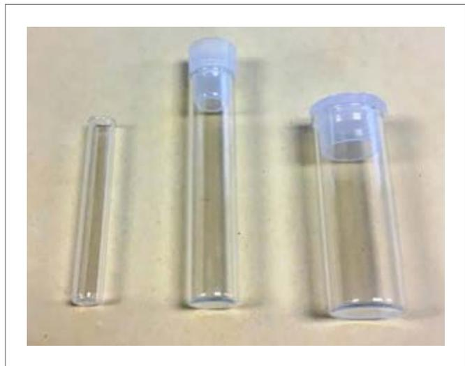
Figure 2. Disposable sample vials for NIR transmission measurements.
