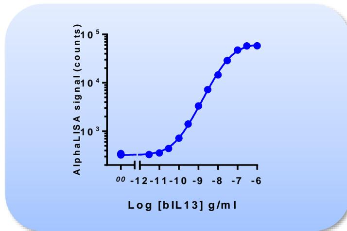
Figure 1. Typical sensitivity curve in AlphaLISA HiBlock Buffer. The data was generated using a white Optiplat<sup>TM</sup>-384 microplate and the EnVision<sup>®</sup> Multilabel Plate Reader 2103 with Alpha option.
