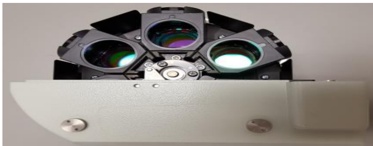
Figure 2. Place the epi-filter turret upside down and loosen the screw that is holding the Texas red filter in place. Slide the filter up to remove.
