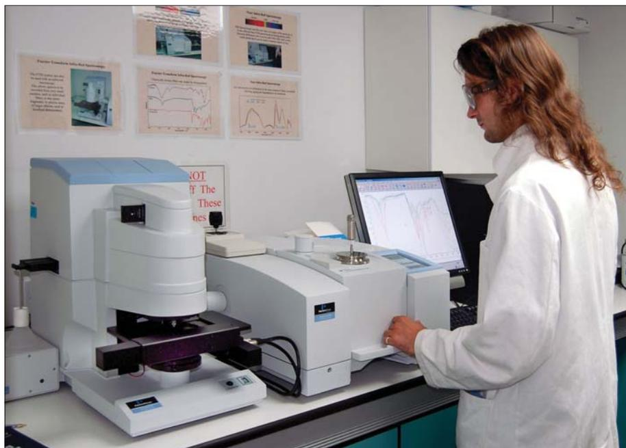
Figure 2. Paul Garside examines textile samples with the PerkinElmer Spectrum One spectrometer fitted with a modified PerkinElmer Universal ATR accessory and to the left, a PerkinElmer AutoIMAGE microscope.
