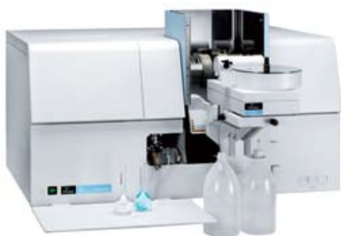
Figure 1. PerkinElmer AAnalyst 800 Atomic Absorption Spectrophotometer.
