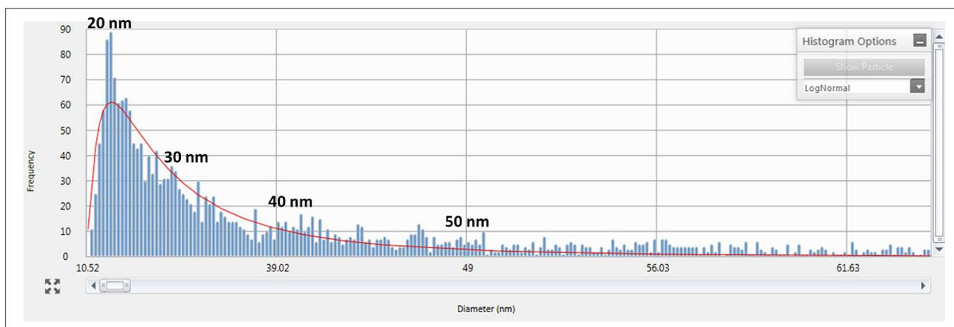
Figure 1. Histogram showing particle size distribution of a typical CMP slurry.
